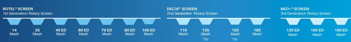
\*SV-Special Screen with 45 angle mesh for Geometrical Design | ED-Extra Thick Extra Durable
